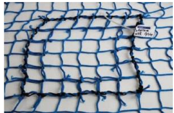
Figure 2. Repair patch attached by lacing repair twine through the perimeter meshes and using cable ties on the inside meshes
