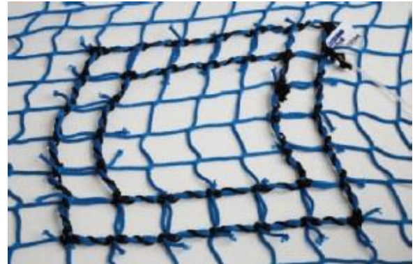
Figure 1. Repair patch attached by lacing repair twine on the inside and perimeter meshes
