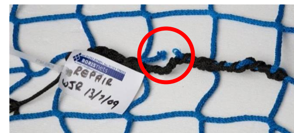
Figure 3. Single strand repair, highlighting the torn strand
