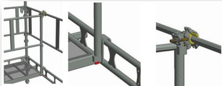
HAKI MK2 – P-Frame before 2018. Addition of Adapter 35 and Double Coupler (Fig. 5)
