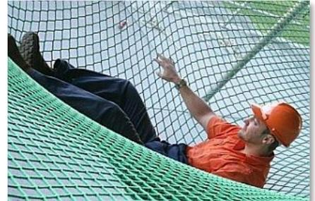
For these reasons, it is not possible to predict the performance of the net should it be subjected to additional loadings in the future. BS EN 1263/1 stipulates that nets should be checked by a competent person after loading. This is generally considered to be the manufacturer (not the installing company) and due to the logistics of this, FASET recommends that safety nets should only be loaded once.
