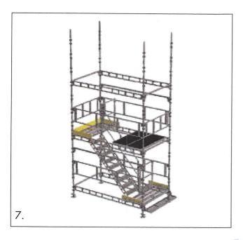
7. Lift up the erection platforms to the next level and install the next set of standards, transoms and ledger beams for the third lift. Install toeboards.
