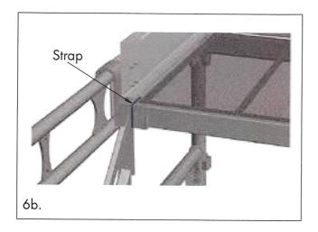
**6b.** For traditional stair tower, in the event of anticipated excessive wind conditions, it is recommended that the flights are secured (at the outboard top edge) by the use of a suitable, disposable strap.
