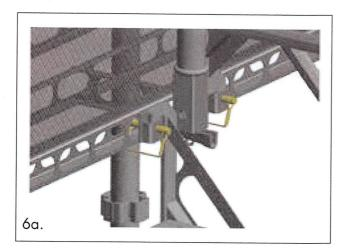
**6a.** The stair flight should be locked in the landing using locking pins (2 per flight).
